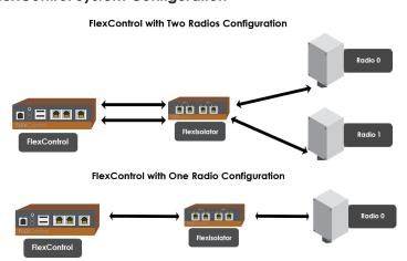
A typical FlexControl system configuration consists of one FlexControl and two Radios with a FlexIsolator. The system can also consist of a FlexIsolator and a Radio. The FlexIsolator offers electrical isolation up to 2,500 V, surge protection up to 12 A, and AC power cross protection.
